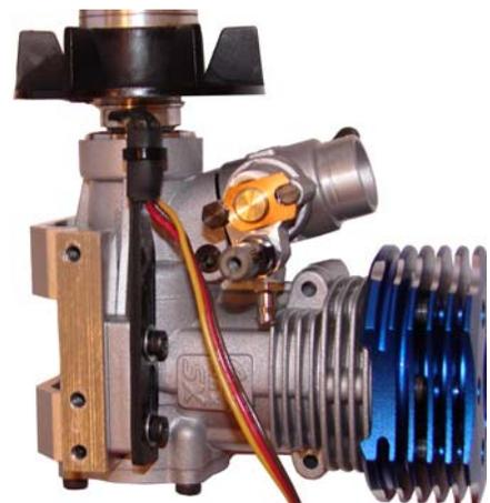
RPM sensor mounted on motor
