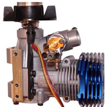
RPM sensor mounted on motor
