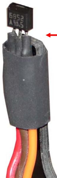
Heat shrink wrap on RPM sensor and bracket
