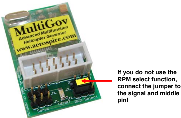
Figure 5. Connecting the jumper to the “RPM Select” input
