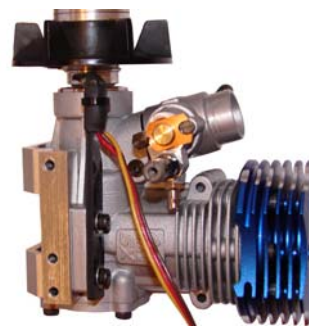
Figure 3. RPM sensor mounted on motor
