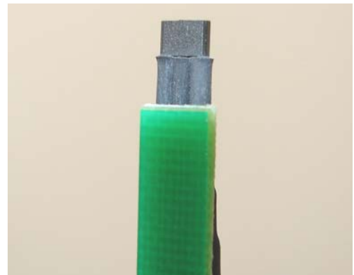
Figure 1. Use green bracket to bend sensor 90 degrees
