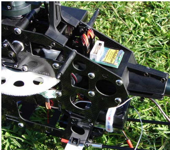
Figure 7. Connecting the jumper to the “RPM Select” input
