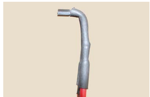
Figure 2. Bent sensor – writing on chip faces up (is on top)
